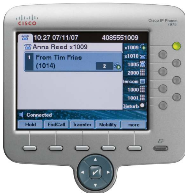
Figure 2. Close-Up of Display and Lighted Line Keys
