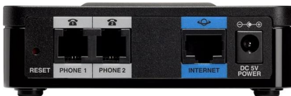
Figure 2. Ports on Cisco SPA112 ATA 2 Port Adapter
