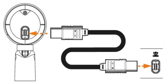
**Note:** Depending on the model of your LifeSize video communications system, the camera symbol appears either above or below the port on the codec.
