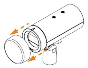
Removing the lens cap also exposes the status LED and the infrared (IR) sensor.
