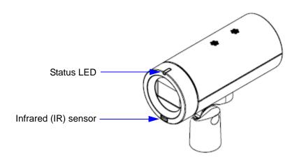
The IR sensor detects signals from the LifeSize remote control up to eight meters (26 feet) away when you use the remote control within two meters (6.5 feet) to the left or right of the front of LifeSize Focus. If you use the remote control directly in front of LifeSize Focus, the IR sensor detects the signal up to 14 meters (45 feet) away.
