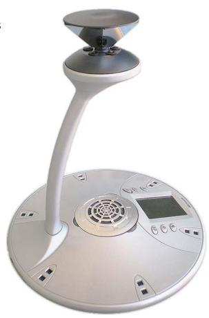
When connected to the telephone network, Microsoft RoundTable can also be used as a standard speakerphone for audio conferencing.
